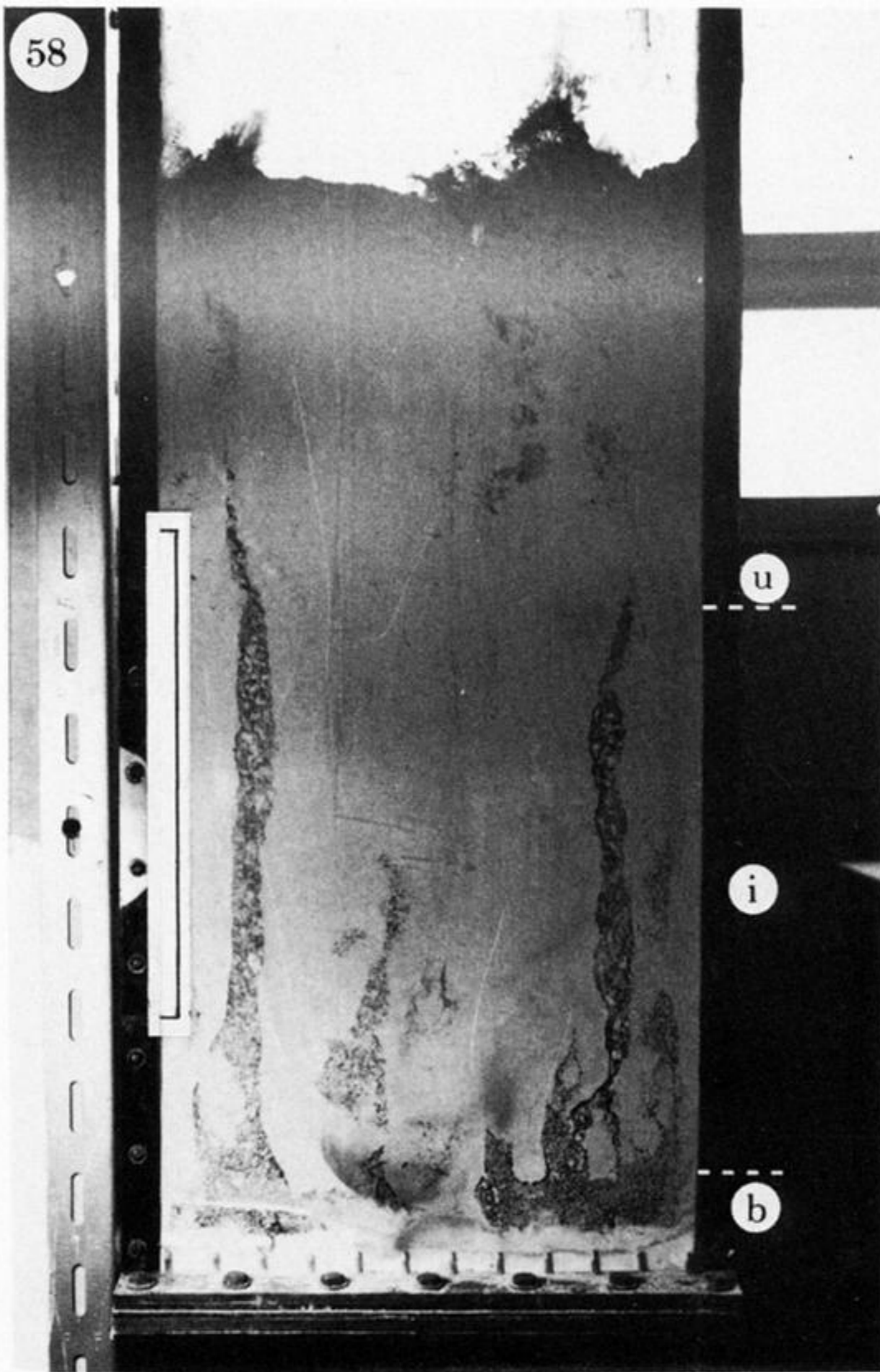
FIGURE 58. Fluidized ignimbrite sample (Wilson 1980, figure 4), showing the basal (b), intermediate (i) and upper (u) portions of the bed (see text for discussion). Scale bar is 25 cm.
